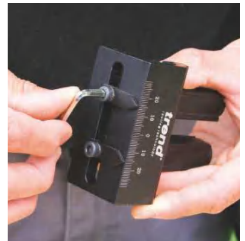
▲ Pic.10 Trend's Mini Pocket Hole jig was used to provide a strong edge-to-edge joint on the underside of the cover
